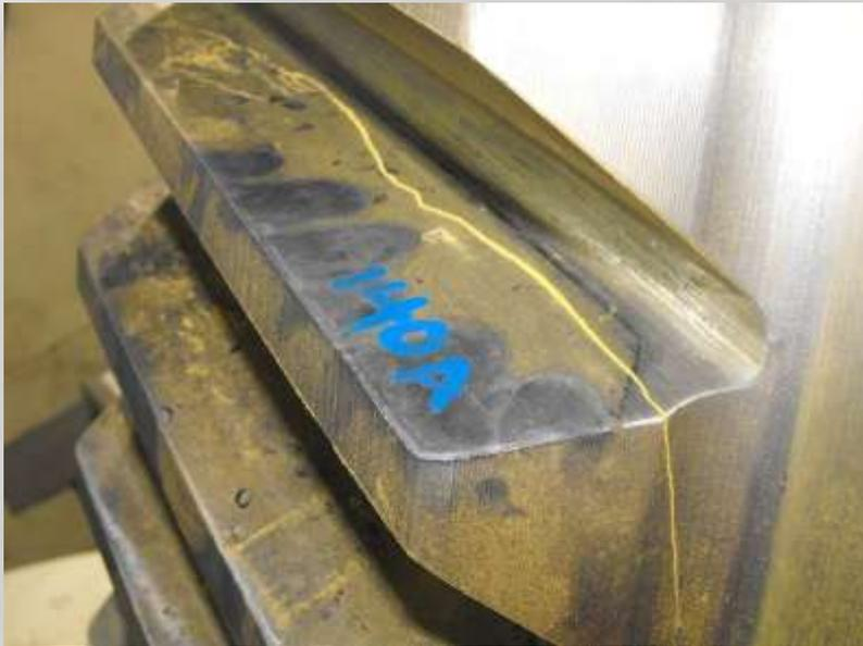
FIGURE 15 – Crack on a Gear Flank
