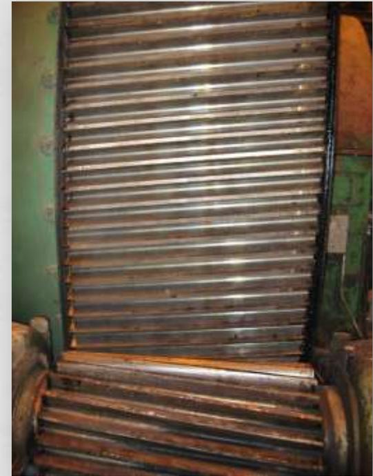
FIGURE 10: Clean Ring Gear and Pinion
