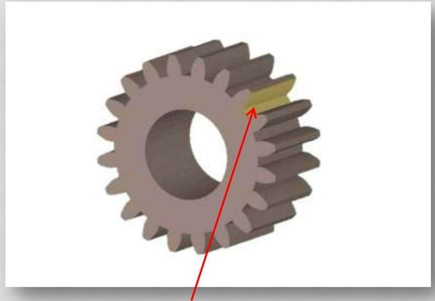
FIGURE 5: Coverage of the ECA Scan
