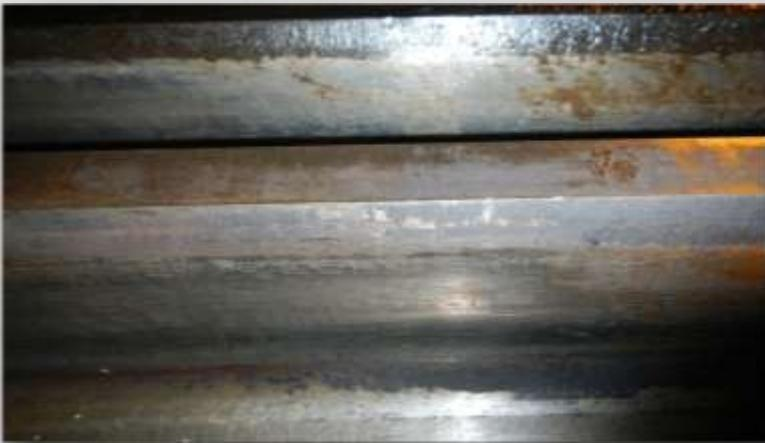
FIGURE 6: Gear flank in good condition
