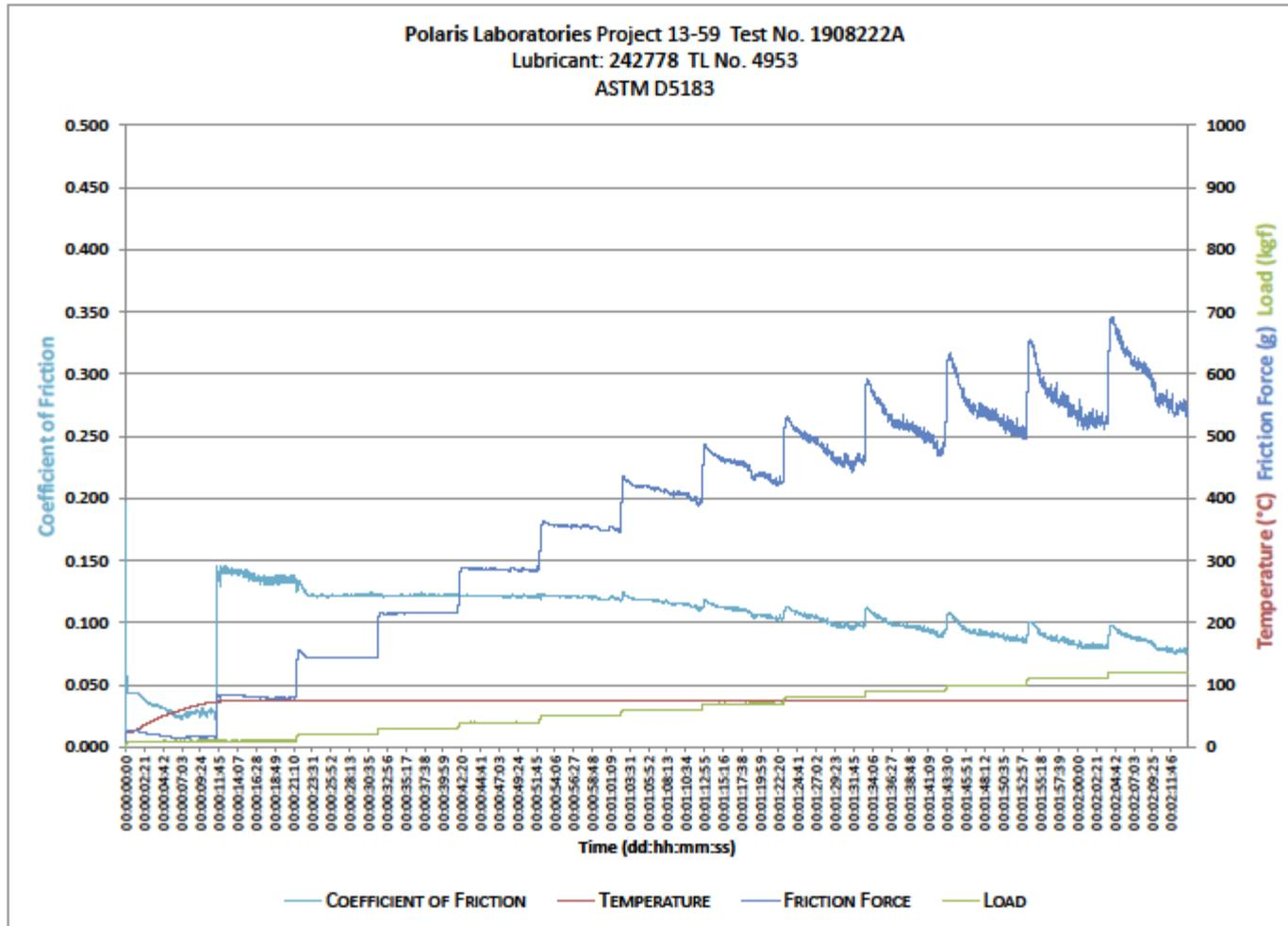
FIGURE 11: ASTM D5183 Results
