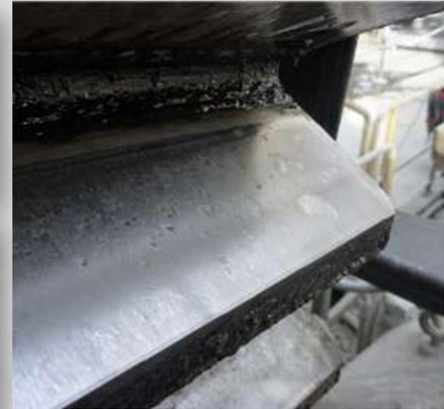
FIGURE 12 – Crack found in the root that could not be visualized. C-Scan image in Figure 13
